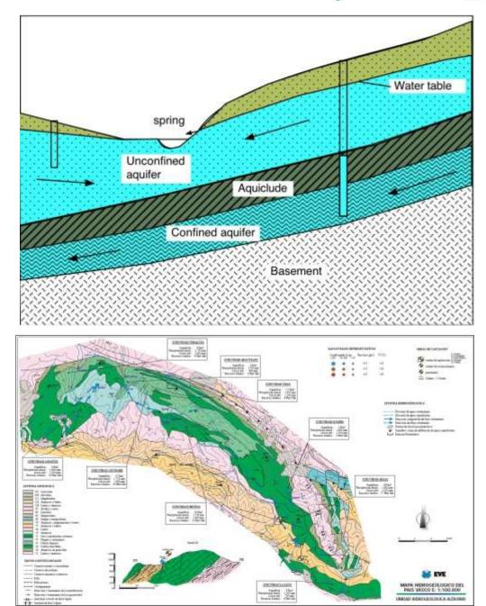
Figure 2. (top) Hydrogeology, aquifer diagram
