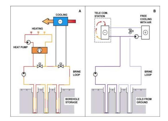
Fig.7. Principal system for combined heating and comfort cooling (A) and for process cooling (B)
