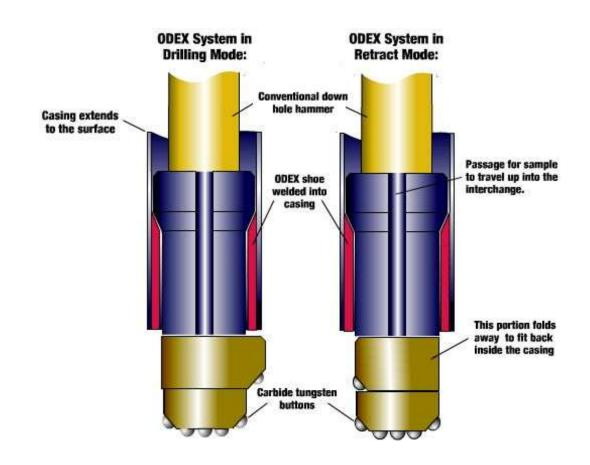
Figure 6. Principal and equipment for the ODEX drilling method
