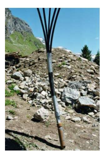
Figure 1. BHE on a decoiler during the first density test using air (picture: Polydynamics Engineering Zurich)
