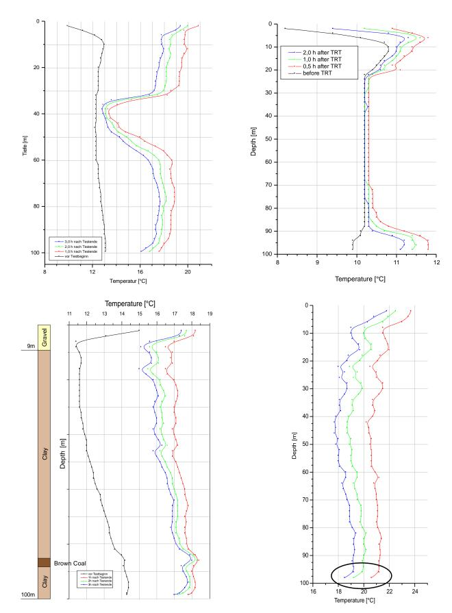
Figure 15: Features as elucidated by temperature log before and after TRT: Influence of groundwater-flow (top left), poor or non-existent grouting (top right), presence of a low-conductivity layer (bottom left), prove of final depth (bottom right)
