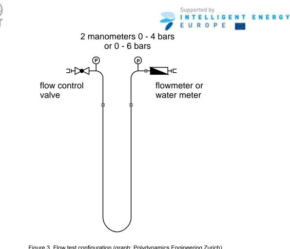
Figure 3. Flow test configuration (graph: Polydynamics Engineering Zurich)
