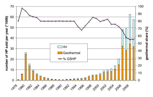
Figure 4. Development of heat pump sales in Germany (after data from BWP and GtV-BV)
