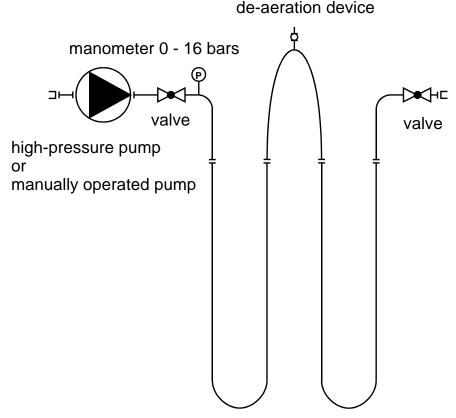
Figure 5. Leak tightness test configuration (graph: Polydynamics Engineering Zurich)
