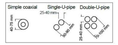
Figure 1. Cross sections of three most frequent BHE types
