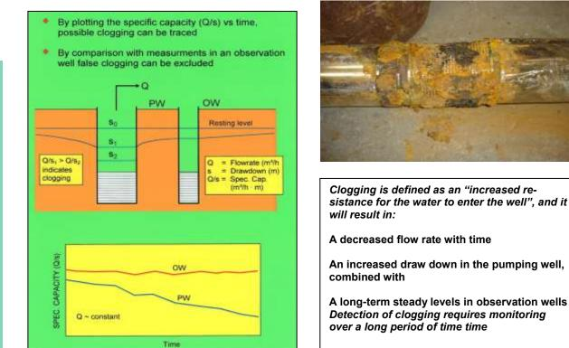
Fig. 2. By using a monitoring program clogging can easily be traced in an early stage. On top right, a clogged inlet screen on a submersible pump, cased by iron precipitation.
