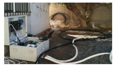
Figure 4: When setting up a TRT, the length of connection pipes between BHE and TRT should be as short as possible, and the BHE and connection pipes must be well insulated; to the left a correct setup, to the right an inappropriate setup from a SE-European site
