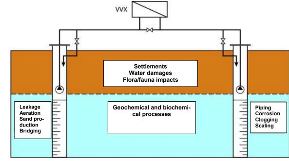
Fig. 1. Potential technical and environmental problems related to open loop systems
