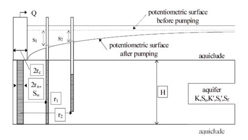
*Figure 4. Hydraulic properties of an aquifer is obtained by a longer pumping test where a number of observation wells or pipes is used to determine the shape of the draw down cone.*
