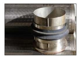
Photo showing a continuous slotted screen together with a simple type of packer used for lost filter completions
