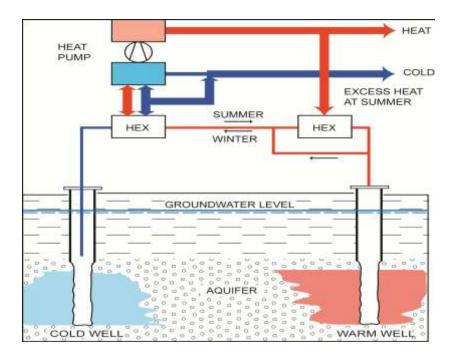
Fig.6. Principal flow chart of an ATES system for heating and cooling
