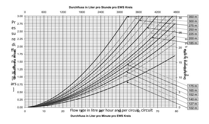
Figure 4. Theoretical maximal allowed pressure drop per circuit of a BHE, tube Ø 40x32.6 mm (graph from SIA 384/6 (SN 546 384/6))
