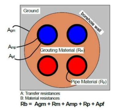
Figure 2. The components of Rb shown in the cross sections of a double-U-BHE
