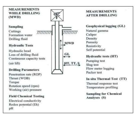
Fig 2. Potential parameters that can be achieved from a test drilling during and after drilling
