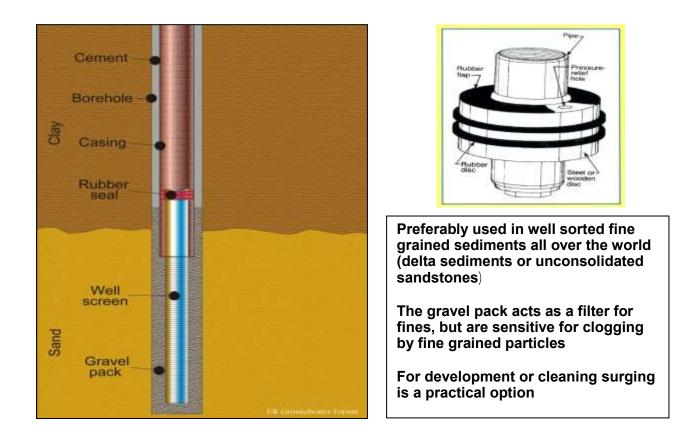
Fig.6. Example of a gravel packed well. On top left a surge block commonly used for development.
