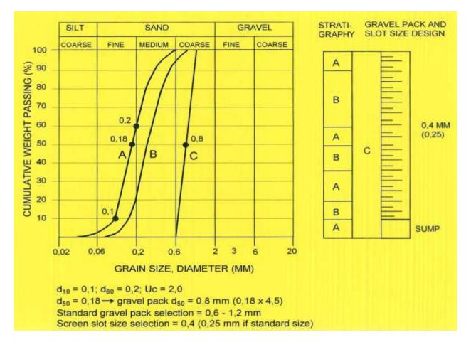
Fig.10. Example on how to select the gravel pack (C) and screen based on the grain size distribution of finest grained layer (A).
