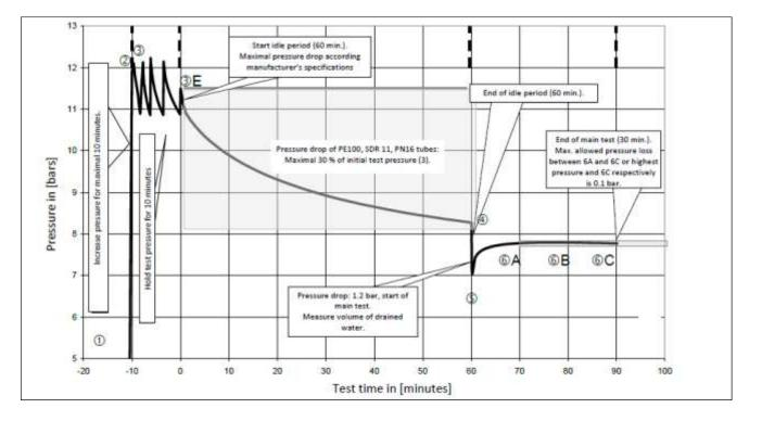
Figure 6. Graphical test procedure (graph from SIA 384/6 (SN 546 384/6)).
