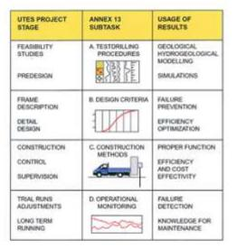
Fig.1. A large scale shallow geothermal system should contain test drillings as basis for design
