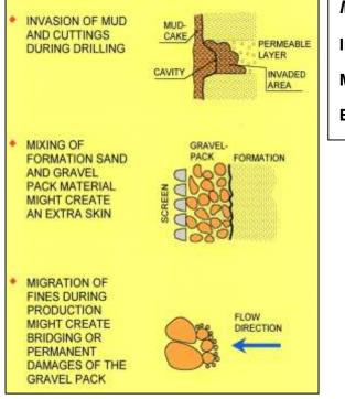
Main causes for particle clogging Invasion of unbreakable mud into the porosity Migration of fines towards gravel packs Bridging in general
