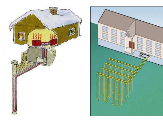
Fig.2. Vertical closed loops applied for a single and a multifamily residential building
