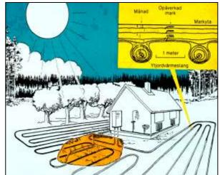
Fig.3. The horizontal loop system that requires large open space to be applied
