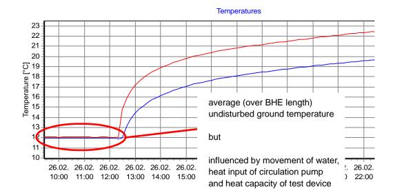
Figure 12: Measurement of undisturbed ground temperature by water circulation without heating
