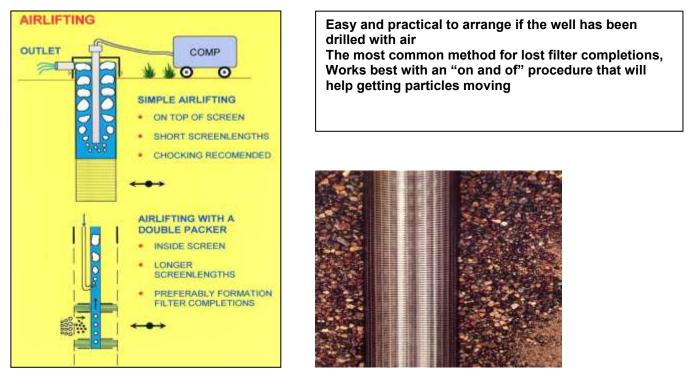
Fig. 5. Air lifting is the most common way for development of formation filter completions
