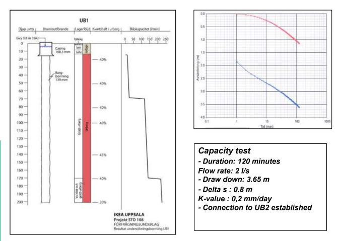
Fig 4. Results from a test drilling for a BTES plant in crystalline rock to IKEA Uppsala, Sweden
