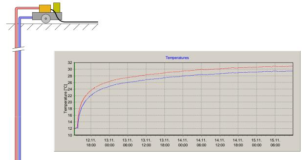
Figure 1: Principle of a TRT and temperature curve of inlet-outlet (good example)
