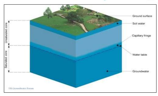
*Figure 1.* The saturated zone defines the groundwater table. An aquifer is in practice defined to be a limited geological formation from which ground water can be pumped by using water wells.
