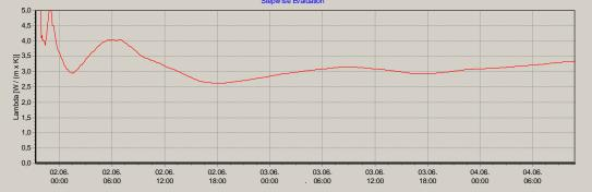
Figure 10: Examples of stepwise evaluation of TRT: Dominated by conductivity, good reliability (top), dominated by advection and not usable (middle), and high fluctuations and low reliability (bottom)
