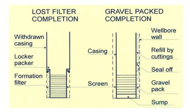
Fig. 4. The two main types of screened wells and their principal design and components
