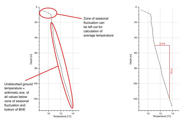
Figure 14: Temperature log and evaluation of average undisturbed ground temperature (left) and geothermal gradient (right, see text)
