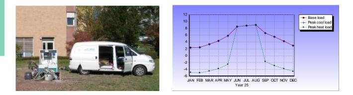
Figure 7. Example of Thermal Response Test for determining ground parameters (left) and calculation of BHE layout using EED software (right)
