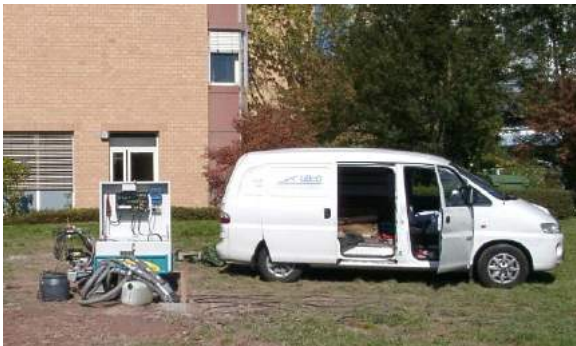
Figure 7. Example of Thermal Response Test for determining ground parameters (left) and calculation of BHE layout using EED software (right)
